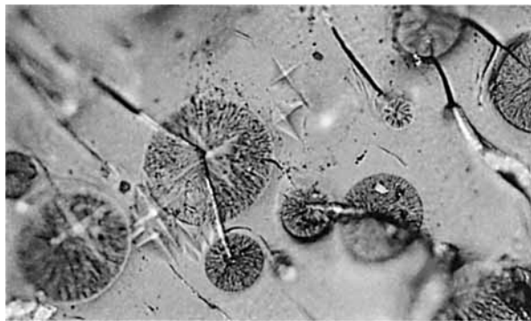
Figure 10 SEM micrographs of the fractured surface of a typical opaque particulate morphology formulation (System B) after microhardness measurements.
